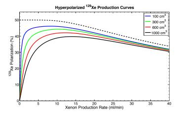
The 9820 xenon polarizer is capable of delivering <sup>129</sup>Xe polarization levels in the range of 35–45% as a function of production rate (1–3 L/h) when operating at the peak laser power. The dashed line shows the typical <sup>129</sup>Xe polarization leaving a 1.5-L cell whereas the color-coded lines depict the collected xenon volume using an effective solid-state xenon relaxation time of one hour.
