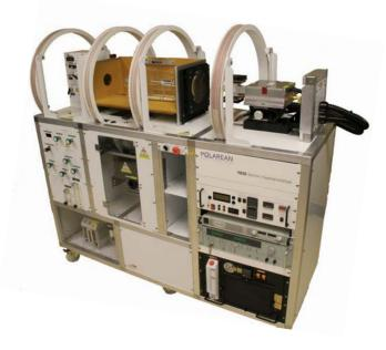
The standard 9820 xenon polarizer configuration comes with a 1.5-L optical pumping cell, a triple-zone temperature control system, custom optics to deliver a highly uniform laser beam across the entire cell length, and a high efficiency cryogenic xenon collection system. The 9820 platform is designed with several expansion options to enhance performance and throughput as new components become available.
